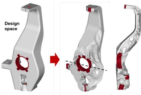
Figure 4: Design space and topology optimisation results on the full knuckle
