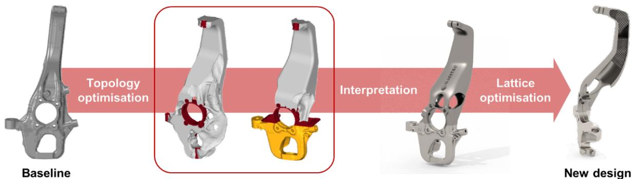
Figure 3: Re-design process for the hybrid suspension knuckle Cobapress/DMLS
