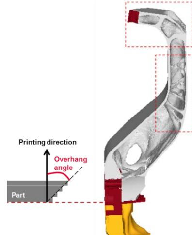
Figure 6: Cross section of the topology optimisation results indicating supports location
