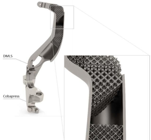
Figure 10: Cross section of the knuckle presenting the lattice optimisation results
