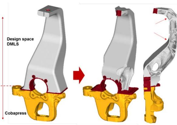
Figure 5: Design space and topology optimisation results on the DMLS part of the knuckle
