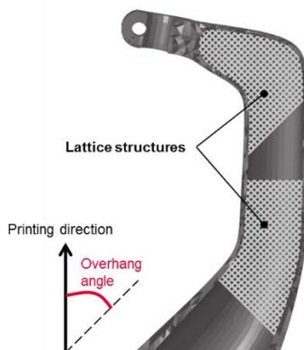
Figure 9: Cross section of the upper part of the knuckle filled with lattice structure
