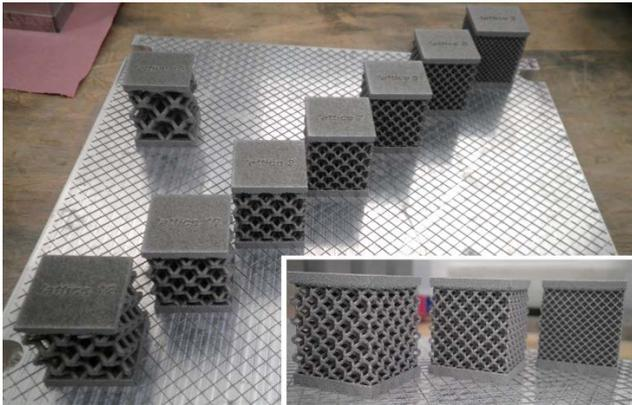
Figure 8: Results of the printing tests of lattice structures
