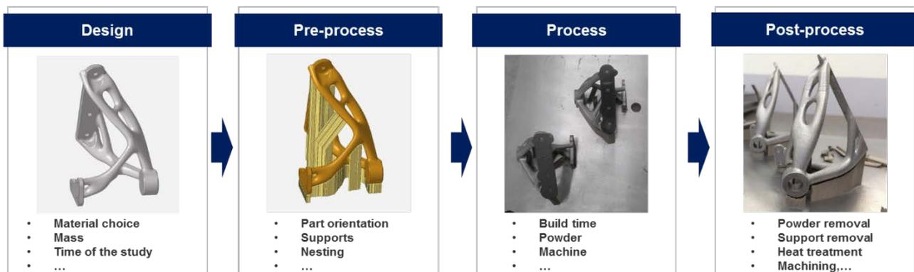
Figure 1: Cost factors in metallic additive manufacturing workflow, a non-exhaustive list
