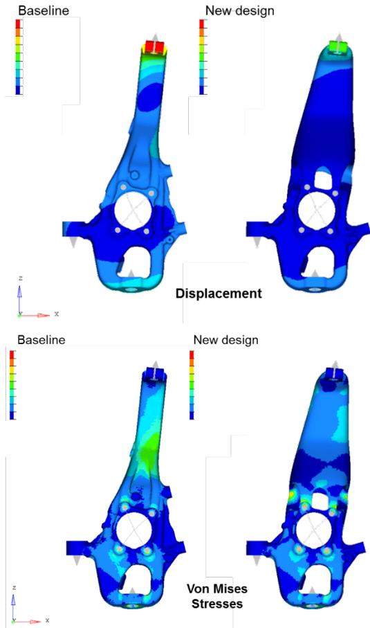
Figure 11: Maximum displacement and maximum Von Mises stresses for the baseline and the new design
